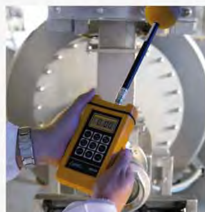
Isotropic sensor for measurement of the electromagnetic field in the area surrounding the device.
