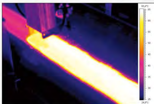
Thermo image recorded during a laboratory test: it shows the temperature distribution on the surface of the treated product coming out from the equipment.
